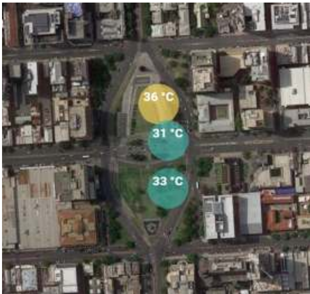
Figure 8. Three sensors in the same park showing a significant temperature difference.
