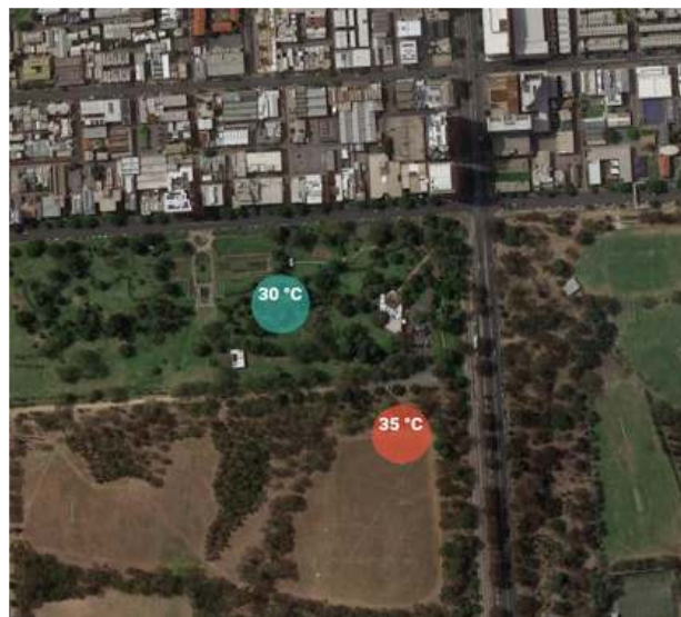
Figure 6. Two sensors in the close proximity showing a significant temperature difference.
